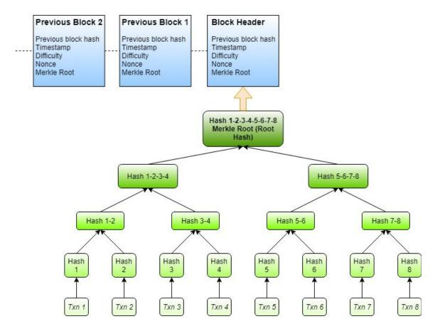
Figure 2: 8 TRX transactions are hashed into the merkle root. This merkle root is then included in the block header, which is attached to the previously confirmed blocks to form a blockchain. This allows for easy and transparent tracking of transactions, timestamps, and other related information.
